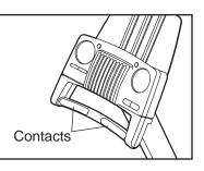
the handgrip pulse sensor, with your palms on the contacts closest to you and your fingers touching the contacts on the opposite side of the handgrip pulse sensor. **Avoid moving your hands.** When your pulse is detected, the heart-shaped indicator in the upper part of the display will begin to flash each time your heart beats. After a moment your heart rate will be shown.
